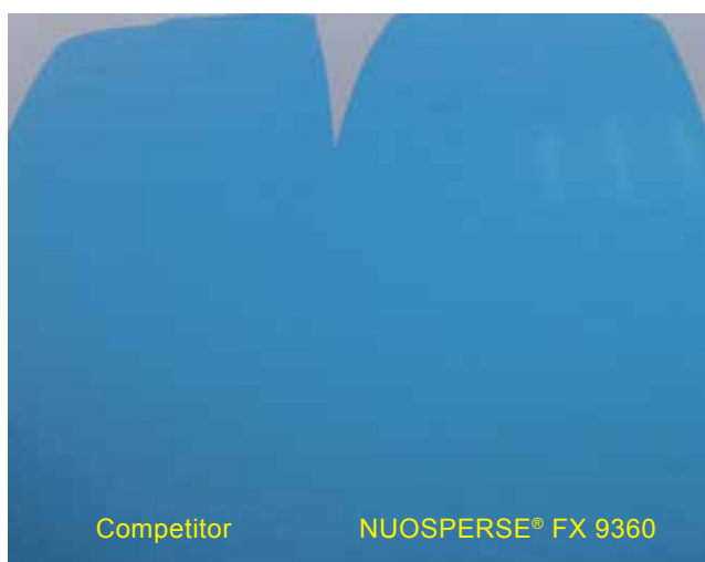
Fig. 27 Metallic paints containing blue colorants dispersed with NUOSPERSE® FX 9360 and the competitive dispersant respectively.
