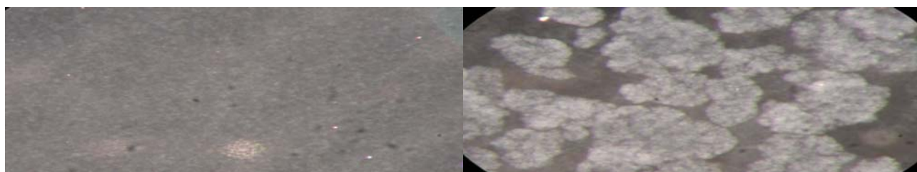
Figure 5. Product with THIXCIN® R, without seeding. Figure 6. Product with THIXCIN® R, showing seeding.
