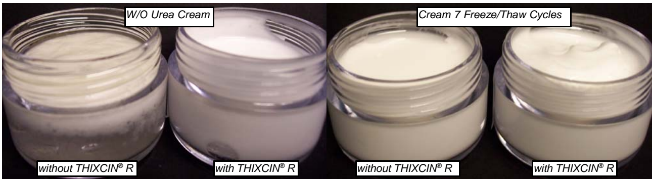
Figure 12. W/O urea cream. Addition of 0.4% THIXCIN® R eliminated all phase separation and gave optimal storage stability performance.
