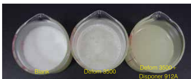
Figure 1 Foam suppression after high speed mixing (top view)
